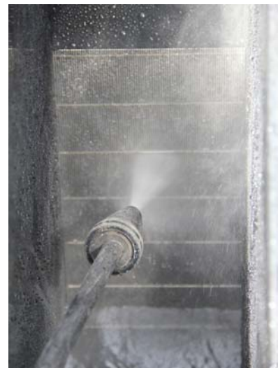
Fig. 23: Cleaning the surface of sieve with high pressure cleaner
