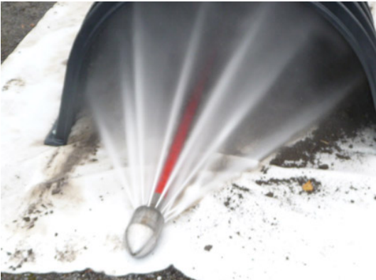
Image 3: Flushing nozzle with reverse conical jets
